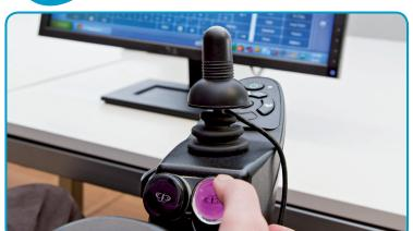
BJOY Ring is an USB device that allows you to convert the joystick of your wheelchair into a mouse to control your computer and compatible tablet or smartphone.
