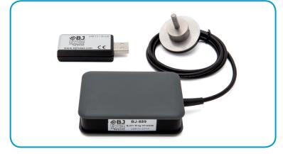
BJOY Ring Wireless offers the same features that the BJOY Ring but without wires. Consists of a **detection ring** with a **transmitter**, that should be placed over the wheelchair joystick, and a **receiver** paired to the transmitter and connected to the device you want to control. Each **BJOY Ring transmitter** can be paired **up to 4 receivers** to be used in different devices or different places.
