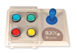
This mouse is based on a sturdy microswitch joystick and big accessible buttons. It is part of the BJOY range of products, which means its hardware can be tailored to each user's needs and capabilities and its operation customized using the BJOY Configurator Software. The BJoy-Stick-C has been especially designed for people with impaired motor skills.
