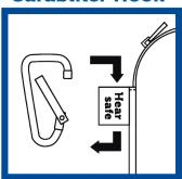
Insert the hook through the tab on the case.
